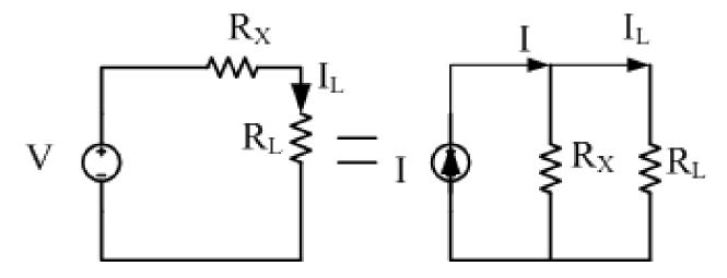
$$I_{L} = \frac{V}{R_{X} + R_{L}}$$
