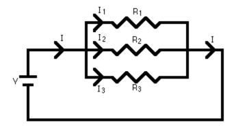
A parallel circuit is shown in the diagram above. In this case the current supplied by the battery splits up, and the amount going through each resistor depends on the resistance. If the values of the three resistors are:
